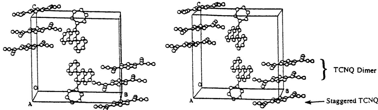
**Figure 1.** Stereoview of a unit cell of  $(\text{TCNQ})_5(\text{DPBT})_2$  showing sections of the TCNQ layer and their relation to the cations. Also designated are the TCNQs which form dimers and the staggered TCNQ in the corner of the unit cell.
